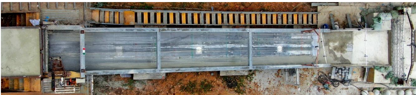
Figure 1. Top view image of the 28 m-long flume with debris material in the storage container
