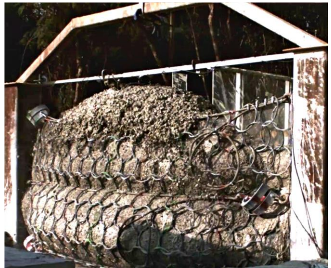
Figure 3. Debris flow run up during impact against a flexible barrier
